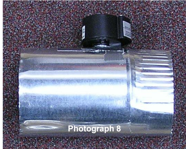
Airflow meter position within the duct fitting
