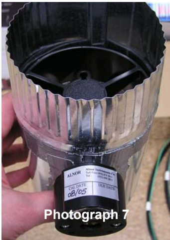
Airflow meter duct fitting
